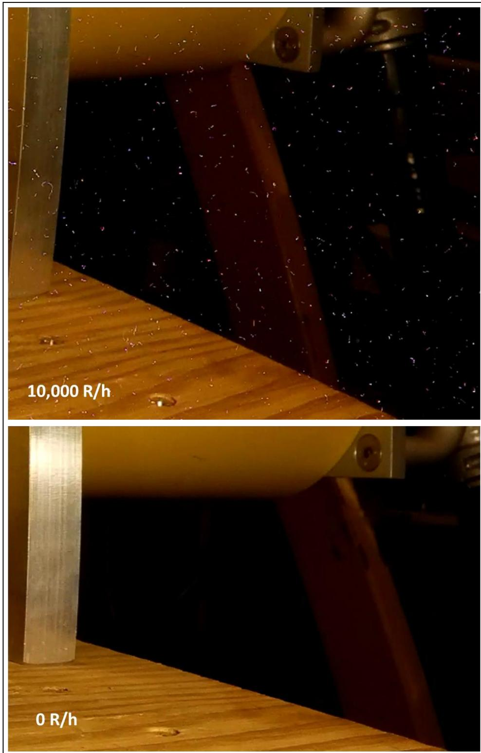
Figure 16. Expanded sections of drone image captured in 10,000 R/h radiation field showing radiation induced noise compared to an image captured in a 0 R/h field
