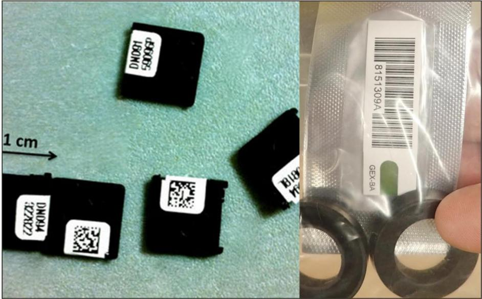
Figure 11. Dosimetry used during radiation testing. nanoDots (left) and GAFChromic HD-V2 film (right)
