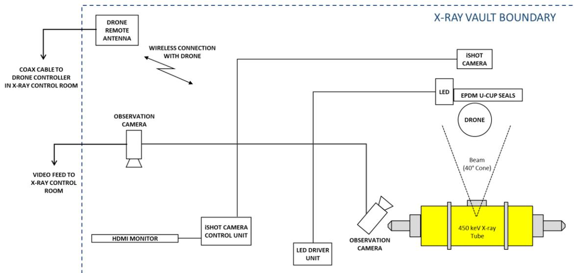
Figure 9. Simplified layout of targets and support equipment for radiation testing
