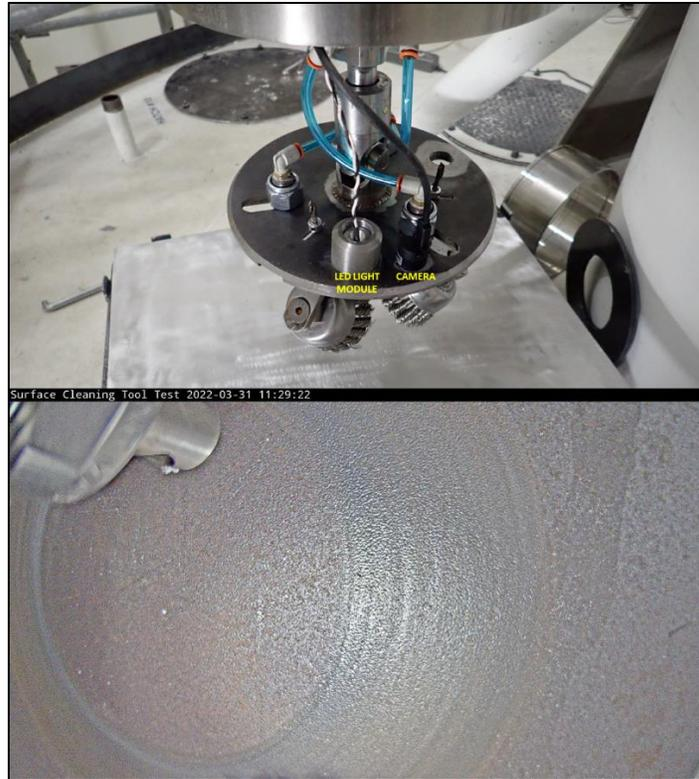
Figure 7. LED light module mounted on surface cleaning tool (top) and image from the camera captured during a mechanical test
