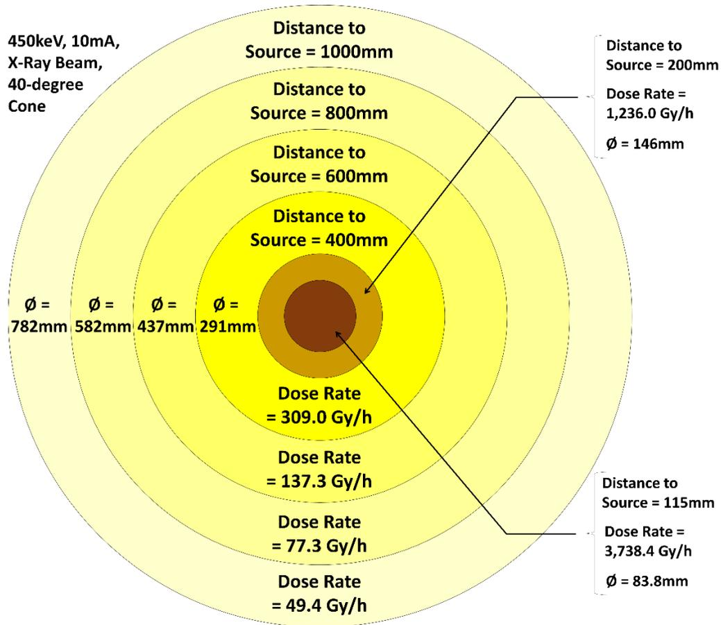
Figure 4. Chart depicting dose rate versus distance to source for 450keV X-ray generator
