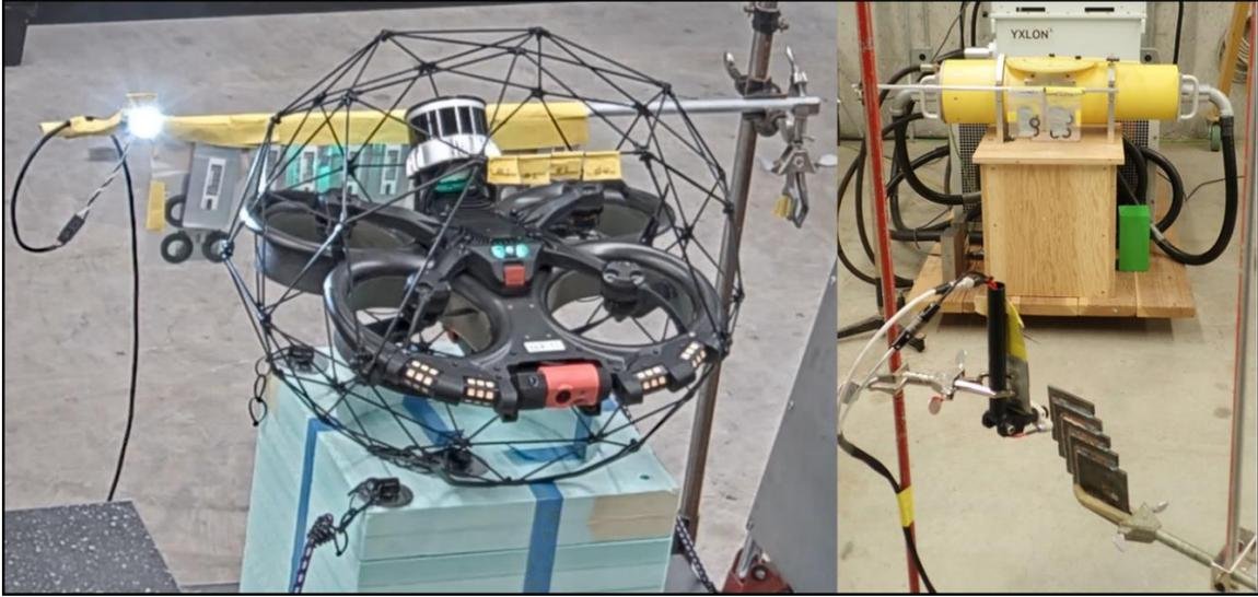
Figure 10. Radiation targets shown with attached dosimetry, Elios 3 drone, LED, and seals (left) iSHOT weld camera (right)
