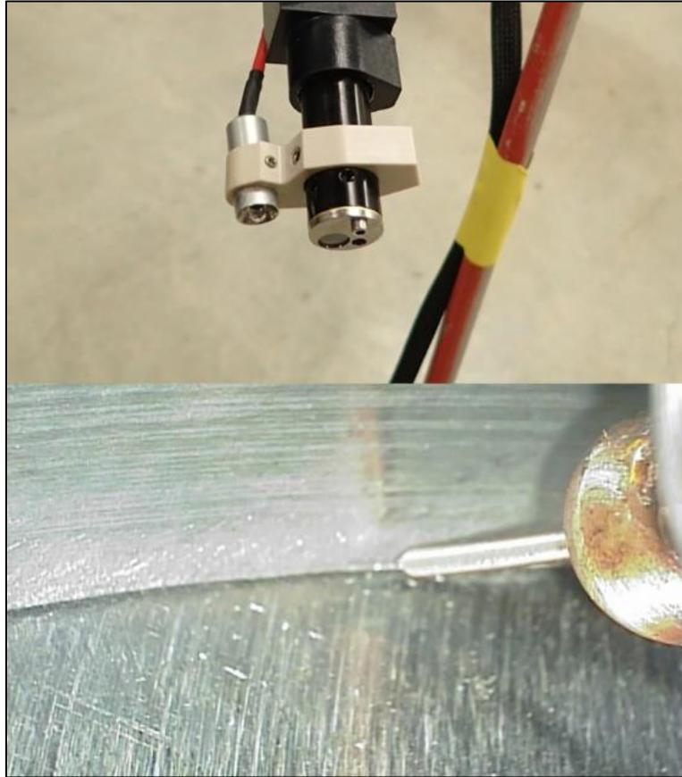
Figure 6. iSHOT weld camera and integrated lamp (top) and pre-weld test image (bottom)
