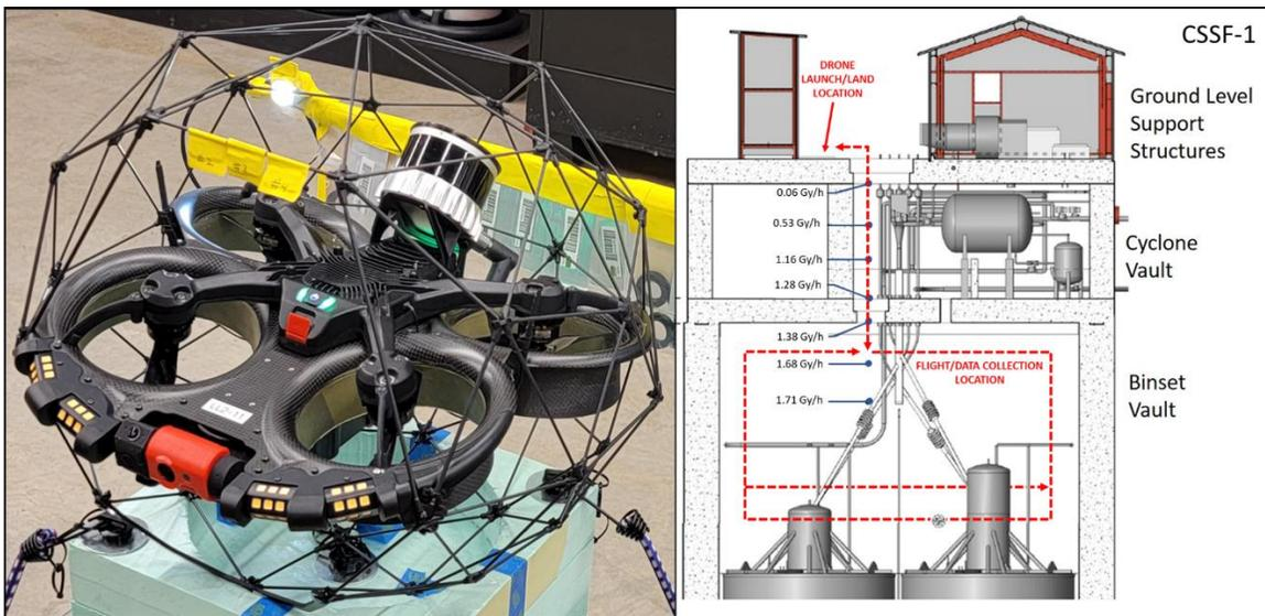
Figure 5. Flyability Elios 3 inspection drone with LiDAR (left) and proposed drone flight path within CSSF-1 vault (right)
