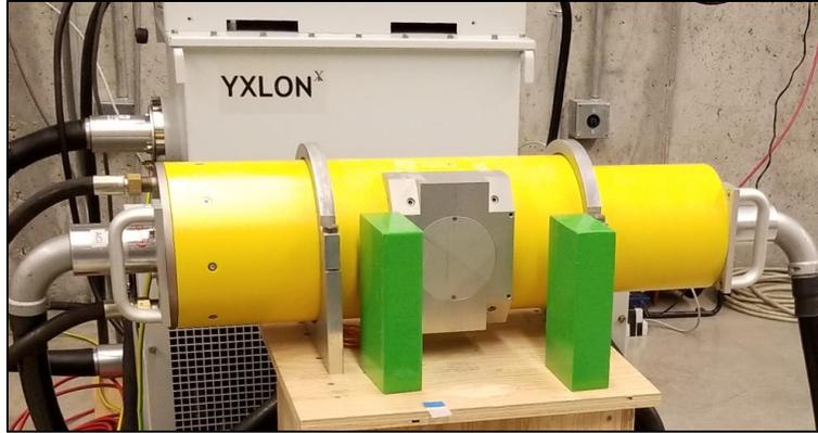
Figure 2. 450keV X-Ray generator used to produce ionizing radiation for testing
