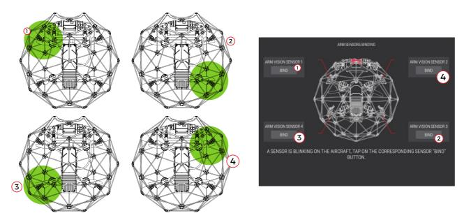
The above illustration is an example of the binding pattern going top-left, bottom-right, top-right, bottomleft. Please note that this is an example, and the binding pattern is random.
