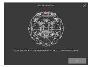
Place the aircraft as shown on the image. Once ready, the aircraft will make the sensor blink one by one. By tapping on the Bind button of the corresponding sensor in the application, the aircraft know the position of each sensor.
