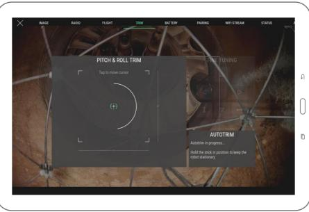
5. New position is then recorded unless the stick has moved too much during the recording. The trim target takes the position of the small cross when recorded. Success is confirmed by the message shown in the Autotrim box on the screen and a sound signal.
