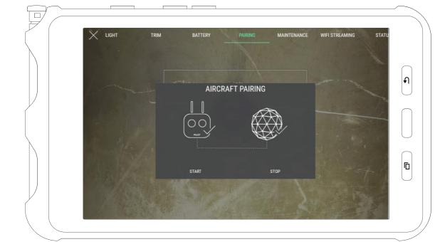
This panel contains the commands to perform pairing operations between a controller and an aircraft.
