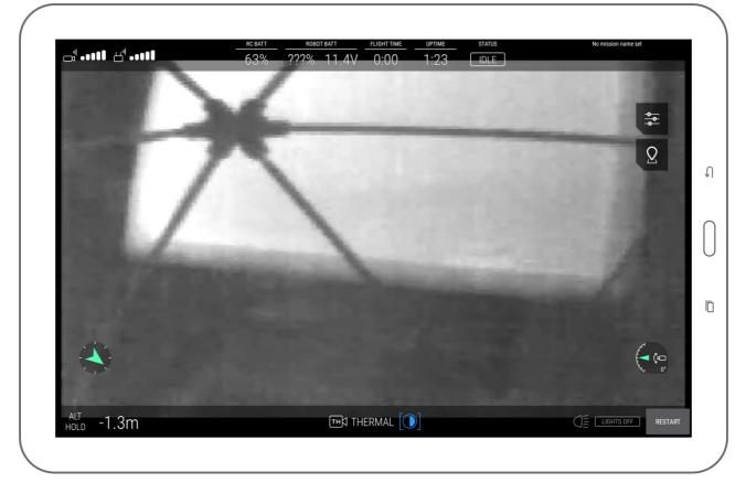
White displays the hottest and black the coldest area on the current frame. The range is always automatically scaled from the coldest to the hottest temperature measured on the current frame.
