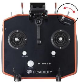
The EV switch sets the camera's exposure value.
