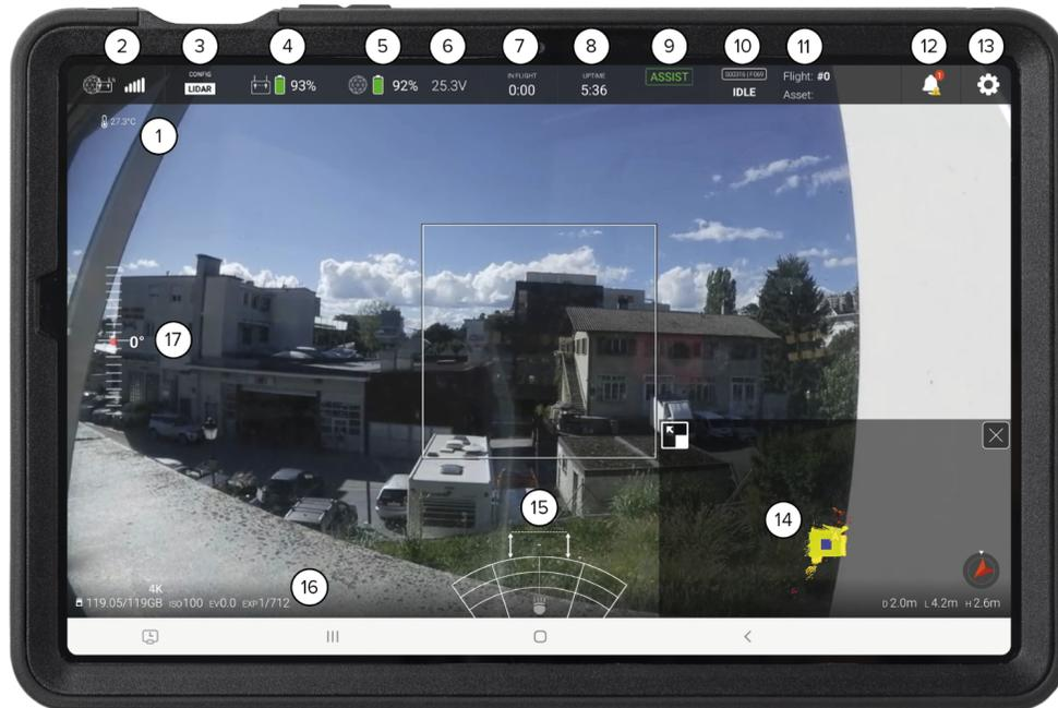
Figure 6.4: ELIOS 3 cockpit
