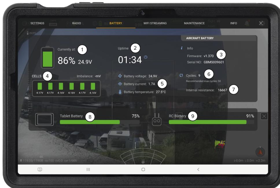
Figure 6.7: ELIOS 3 Battery Panel
