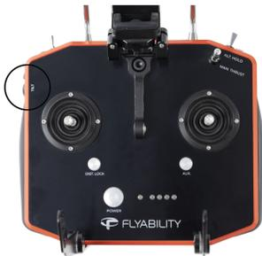
The tilt of the payload can be controlled with the rotary lever on the left side of the remote control. For clarity, the payload tilt angle is displayed on the left side of the tablet's screen during flight.
