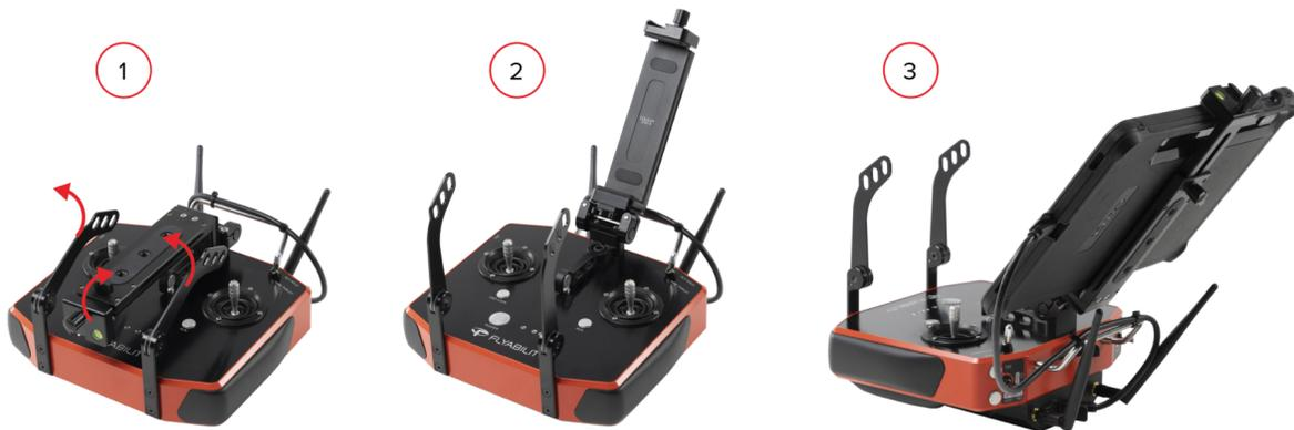
Figure 3.2: Assembly of the GCS
