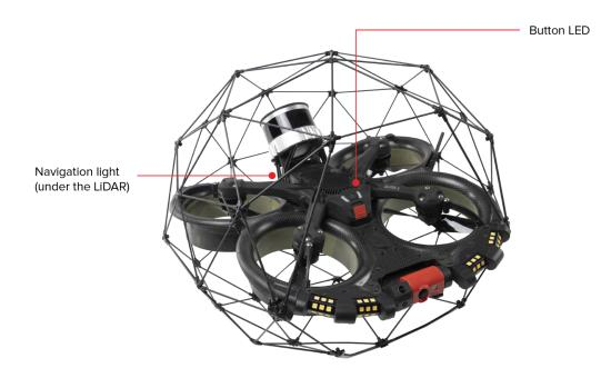
Figure 4.10: Drone Button LED & Navigation Lights
