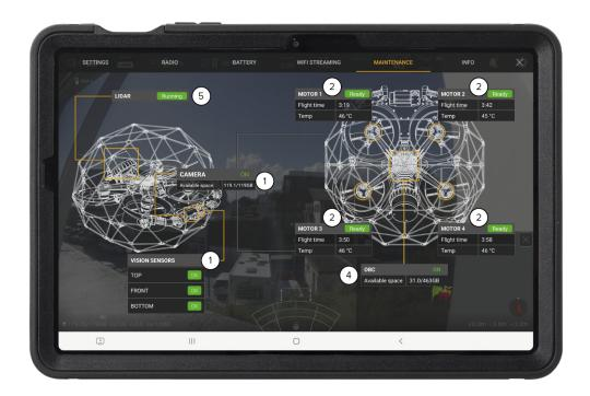
Figure 6.9: ELIOS 3 Wi-Fi Streaming Panel
